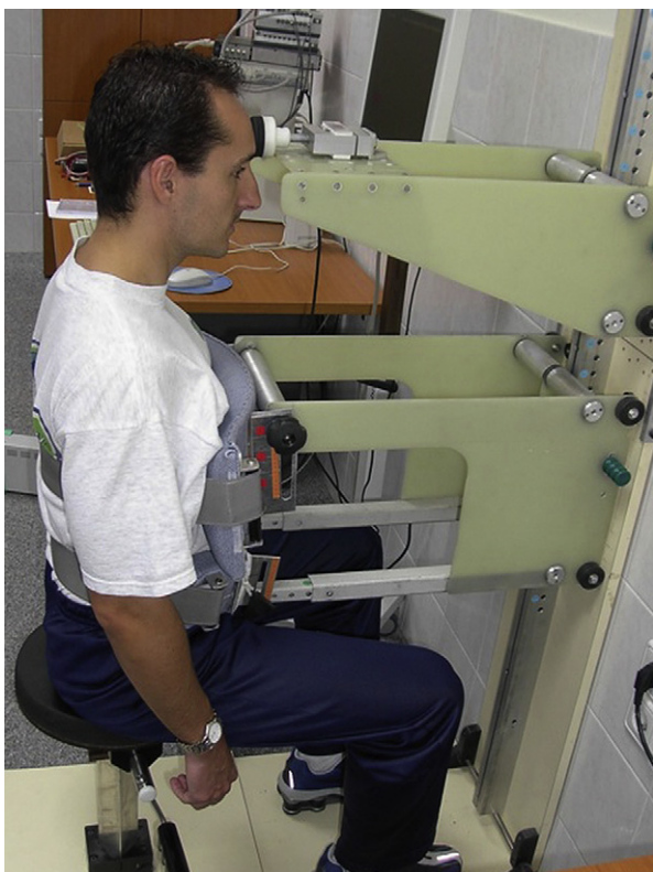
Figure 2 Measuring neck strength during flexion in sitting (Arch. Phys. Med. Rehabil., 2004; 85:1309–1316, with permission from Elsevier).
