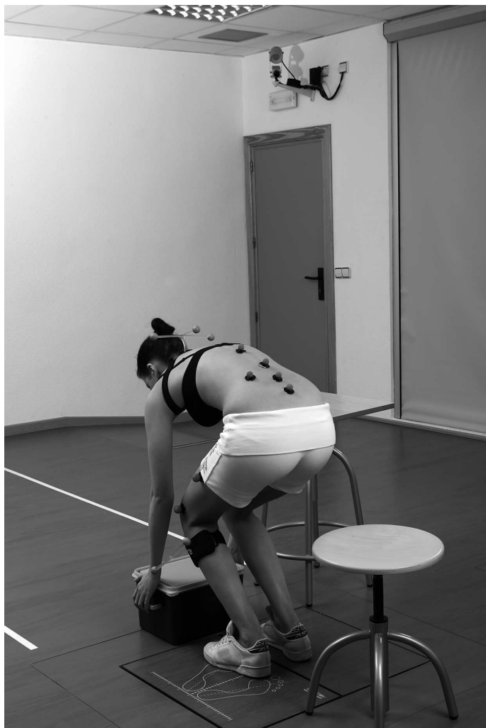
Figure 2. One subject at the moment of getting the box during the lifting task. Note the positions of the reflective markers and the force plates.
