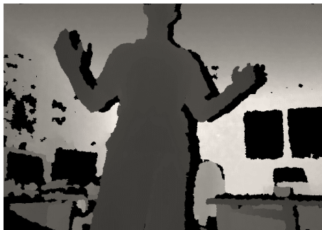
Figure 7. Image of the depth map using the OpenNI tool, from Dyce et al. [9].
