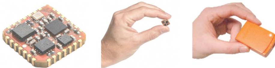
Figure 10 – Image of the sensors that make up an IMU, their size, and then commercially encapsulated, extracted from Xsens ®
