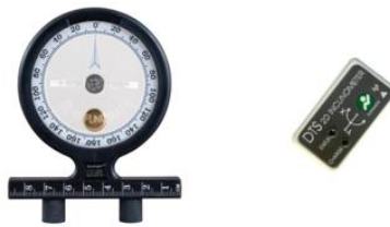
Figure 15 – Baseline® Acu-Angle bubble inclinometer (left) and DTS 2d Noraxon® electronic inclinometer.
