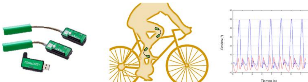
Figure 14 – Example of a commercial wireless electrogoniometer system (Biomec®) used to measure the angle of the knee (blue) and ankle (red) in cycling.
