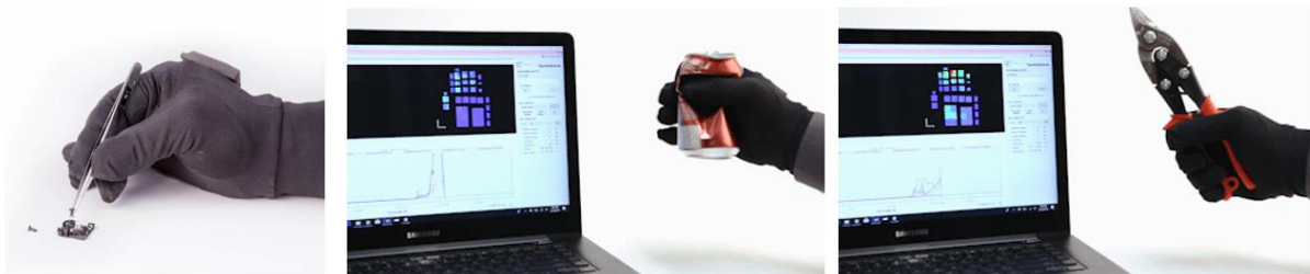
Figure 13 – Example of a pressure analysis system in the Tactile Glove - Hand Pressure Measurement by PPS®, images extracted from https://pressureprofile.com/body-pressure-mapping/tactile-glove
