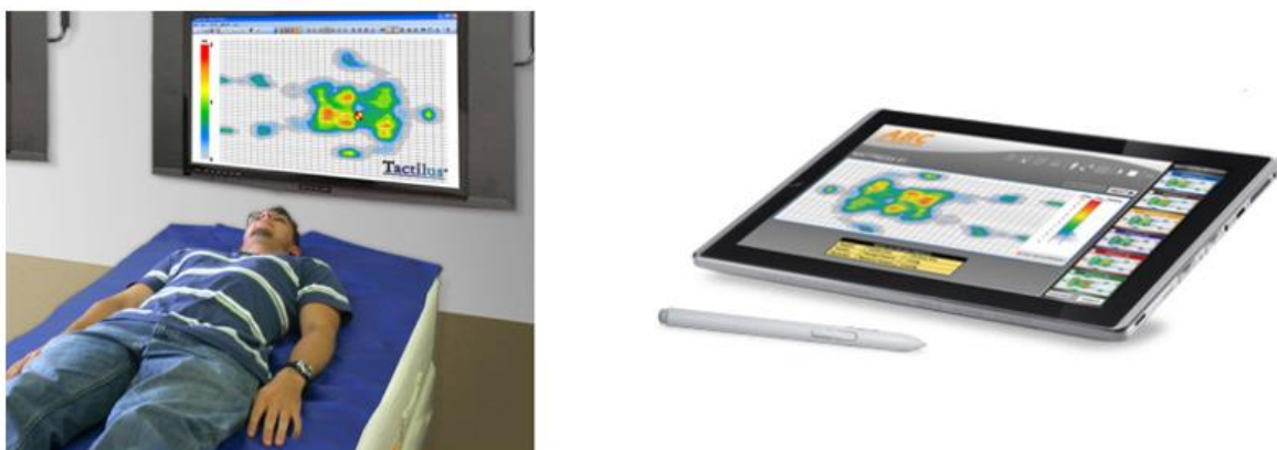
Figure 26 – Example of an analysis of the pressure distribution between person – mattress using the Tactilus Bodyfitter ® system and pressure map (right), images extracted from https://www.sensorprod.com/dynamic/mattress.php
