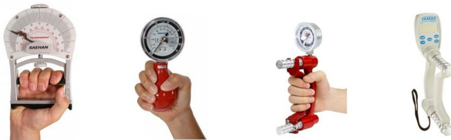
Figure 14 – Examples of dynamometers (left to right): mechanical spring (Saehan Smedley Hand Dynamometer), pneumatic (Saehan hand grip dynamometer), hydraulic, (Baseline® Hydraulic Hand Dynamometers) and digital hydraulic (Jamar Plus+ Digital Hand Dynamometer).
