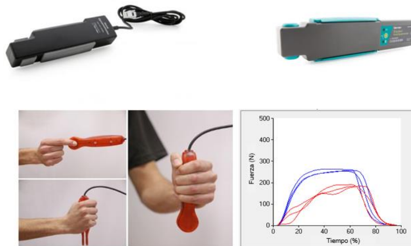
Figure 16 – Example of electronic dynamometers based on strain gauges to measure grip and pinch strength as well as muscle fatigue: (top) wired and wireless dynamometers by Vernier©, images extracted from https://www.vernier.com/products/sensors/hand-dynamometers/ , (bottom) example of the NedVEP/IBV dynamometer associated with the NedMano/IBV software, which provides representations of the repetitions of maximum grip strength of the right hand (red) and left hand (blue).
