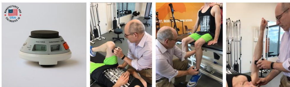
Figure 15 – Example of a manual digital dynamometer: microFET@2 by Hoggan Scientific©, images extracted from https://hogganscientific.com/product/microfet2-muscle-tester-digital-handheld-dynamometer/
