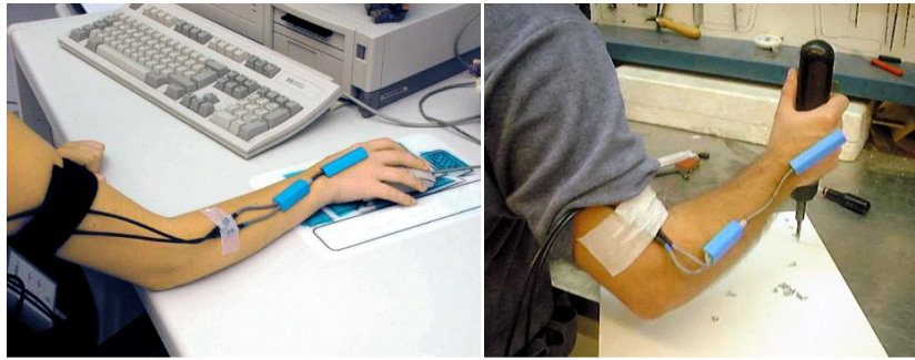
Figure 5: Biomechanical recording of posture during working tasks with electrogoniometers.
