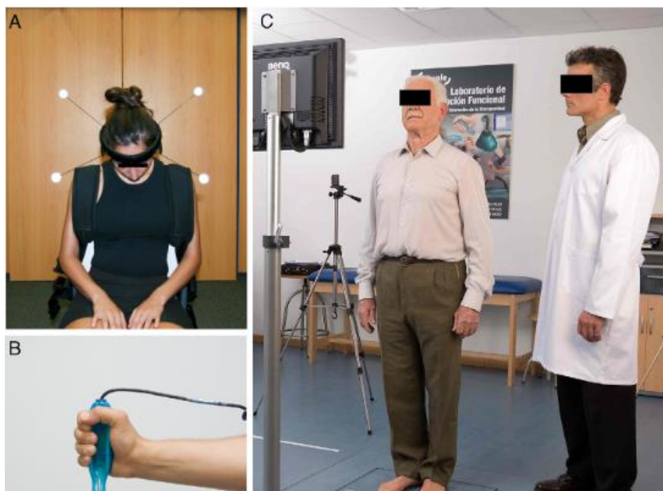
Figure 1: Images corresponding to different biomechanical assessment tests. Cervical motion analysis with fogogrammetry (A), hand grip strength analysis with a hand dynamometer and posturographic assessment with force platform (C), respectively.
