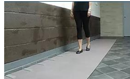
Figure 4. Step length assessment with an instrumented walkway (GAITrite).
