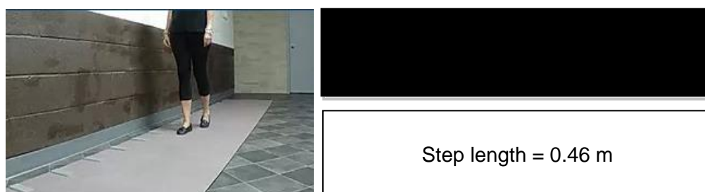
Figure 3 - Step length assessment with an instrumented walkway (GAITrite)
