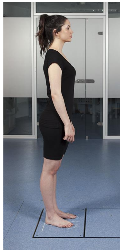
Figure 8. Weight registration on a dynamometric platform prior to gait analysis.
