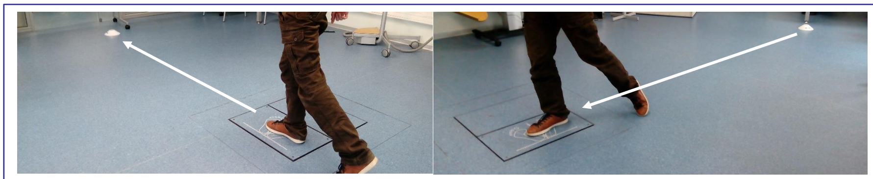
Figure 10. Delimited walkway from gait assessment with dynamometric platform. (Right) Space that allows acceleration before to the step within the platform. (Left) Space for deceleration after stepping on the platform.
