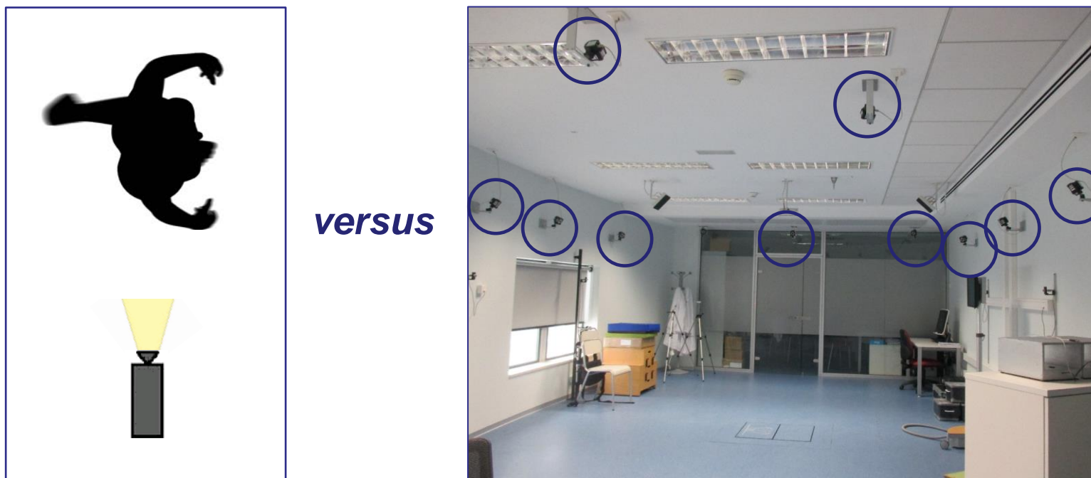
Figure 2. Configuration of cameras for analysis in two-dimensions versus three-dimensions. Medicine Department Lab. University of Valencia
