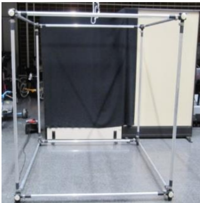
Figure 7. Rigid cubic structure for static space calibration in two-dimensional analysis
