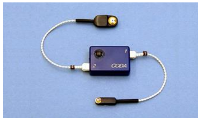
Figure 12: Active markers (Image from J. Richards et al. 2018)
