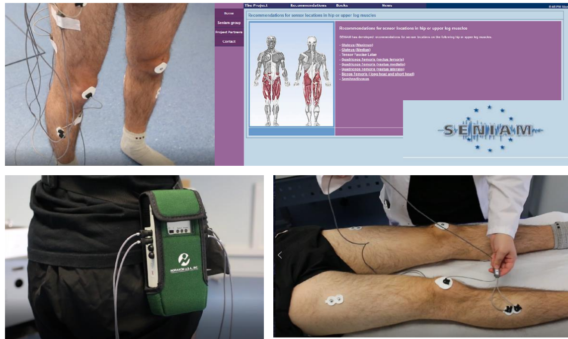
Figure 1 – Surface electromyography system and instrumentation of the lower limb. To determine the instrumentation protocol, the SENIAM guide should be used, which standardizes the location of electrodes in the different body segments. ( www.seniam.org ).
