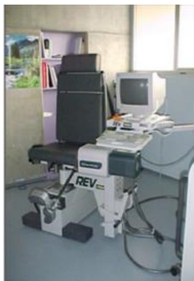
Figure 19. Isokinetic evaluation machine (Source: Internal documents from the Valencia Biomechanics Institute ( Instituto de Biomecánica de Valencia )).
