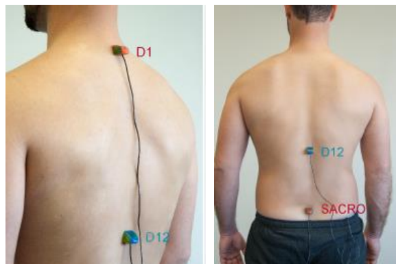
Figure 14. Placing the two electronic inclinometers to measure dorsal (left) and lumbar (right) motion. Sistema NedRangos/IBV (Source: Instituto de Biomecánica de Valencia).
