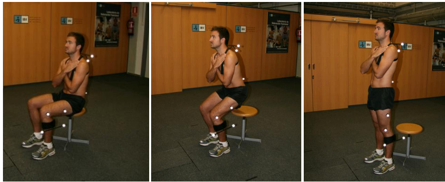
Figure 18. Biomechanical and functional assessment test of the sit-to-stand movement using a photogrammetry system and dynamometric platforms.
